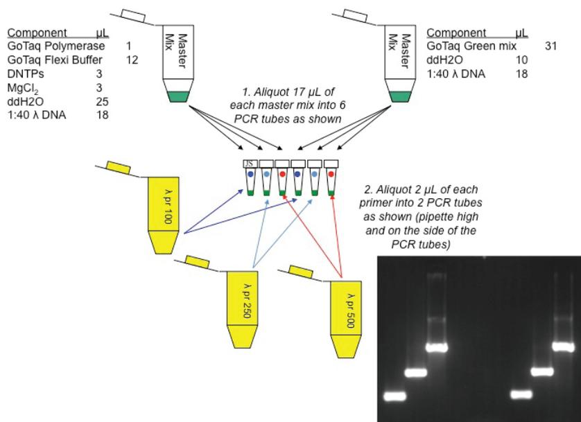
FIGURE 1. Example of master mix setup diagram. Note that this is provided to students as an example—subsequent master mix diagrams are only provided in the instructor materials. Inset shows student generated gel picture of lab.
